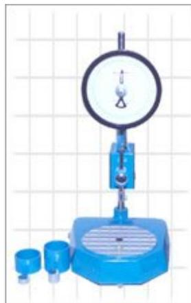
Penetration test for bitumen.
