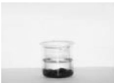
Bitumen coated aggregates kept in distilled water
