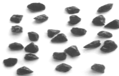
Aggregates kept out side for observation of stripping of bitumen coating
